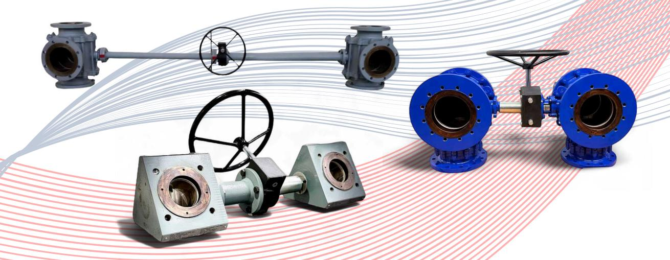
KAVAATA is market leader in Double 3-way valves also known as Double 3-way transfer valves. These valves are manufactured by coupling two "3 Way Ball Valves" together by a rigid/ flexible coupling. A single handle is provided to operate the two valves simultaneously. These types of valves are specially used in Duplex Heat Exchangers and Duplex Filters.
